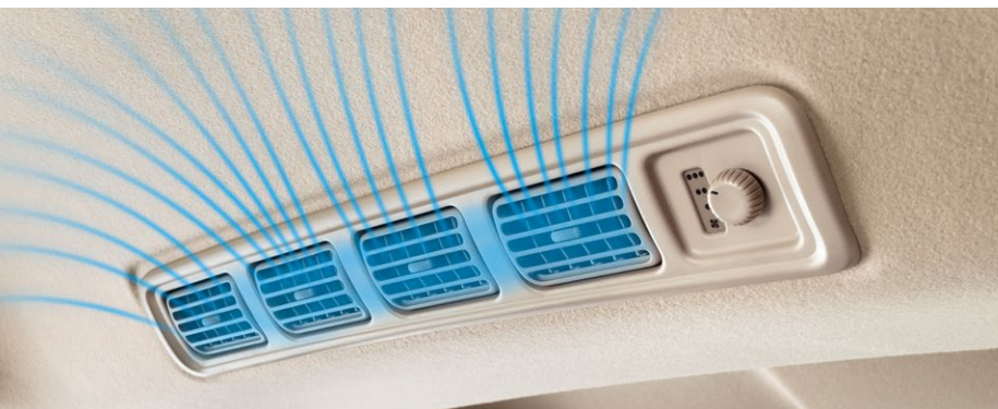
2 ND ROW ROOF MOUNTED AC WITH SPEED CONTROL
